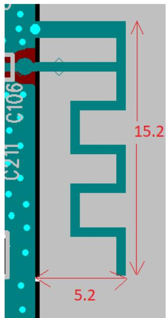
*Figure 1 Physical dimension (mm)*
