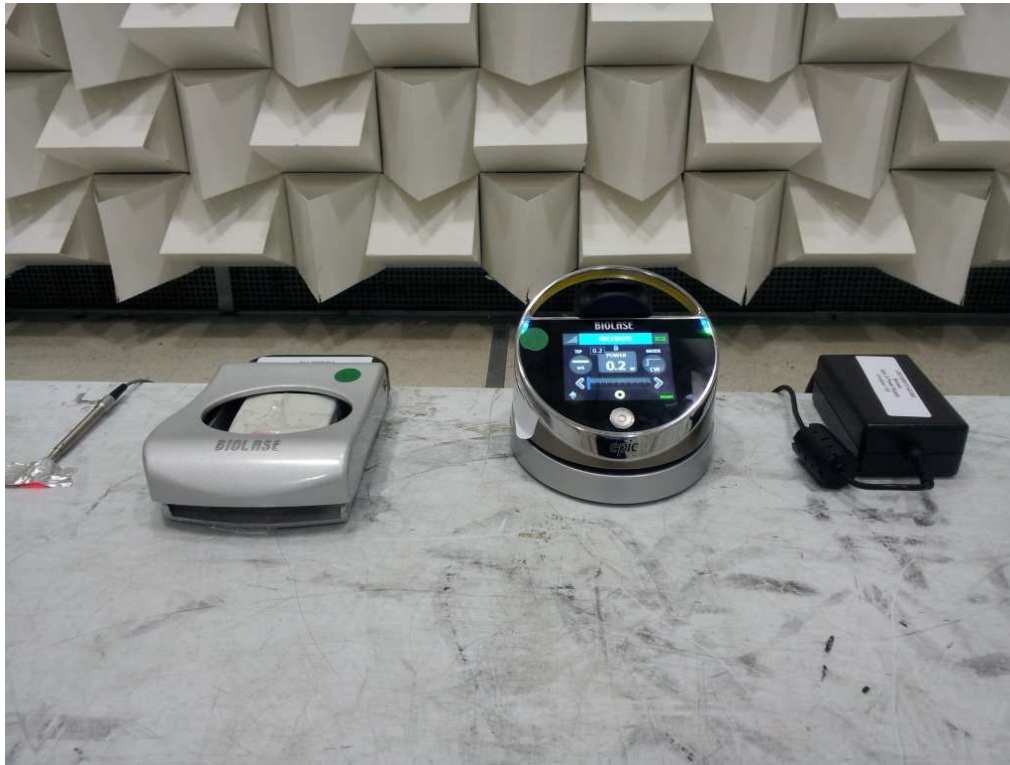
Epic T / Epic S Laser System (front view of product: pictured from left to right, laser hand piece, remote control foot pedal switch (EUT), laser console, and power supply)
