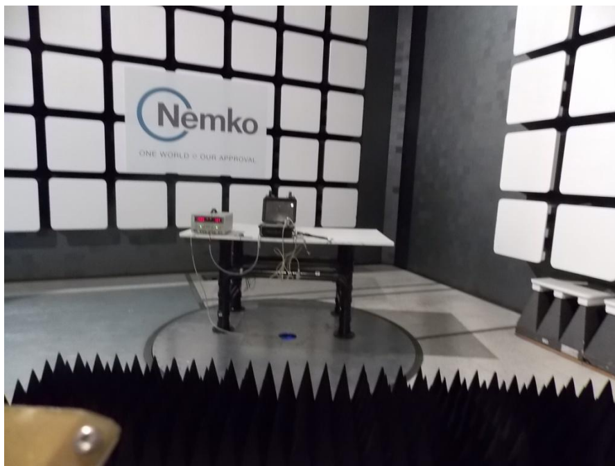
Figure 8.1-4: Radiated disturbance setup photo
