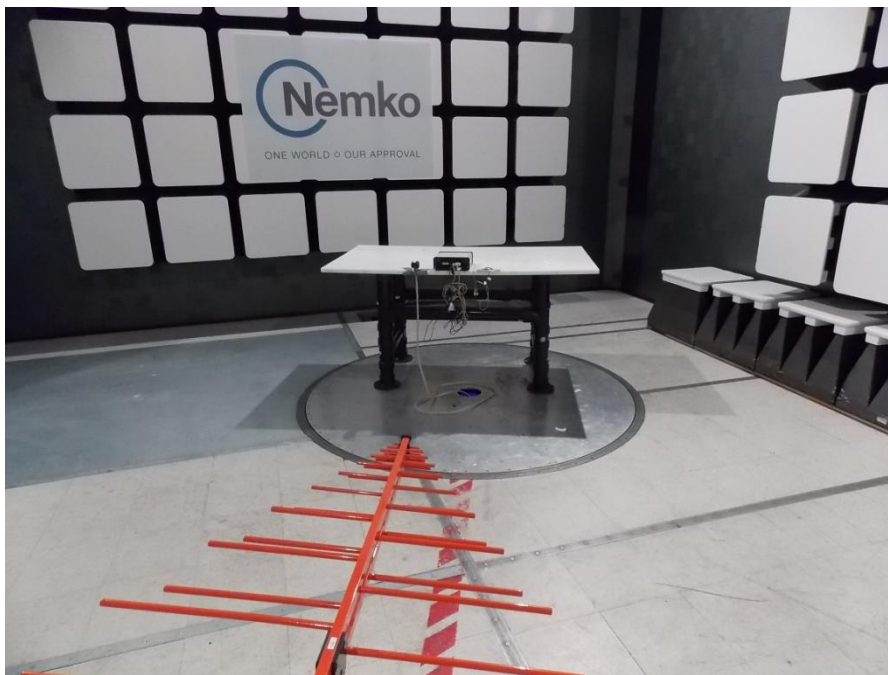
Figure 8.1-2: Radiated disturbance setup photo
