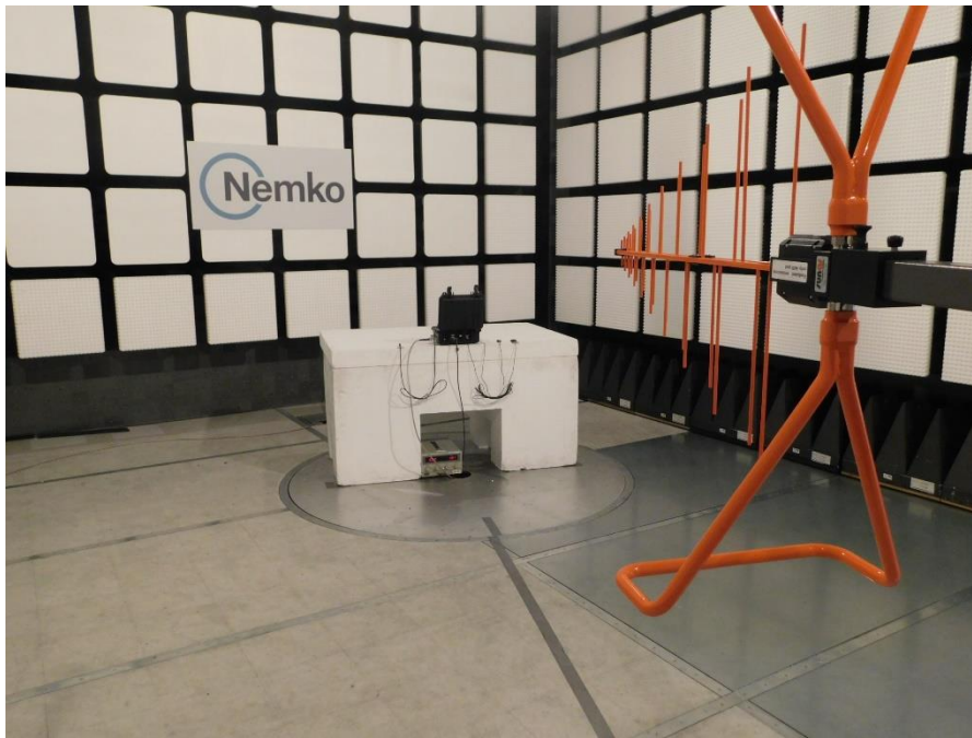
Figure 8.1-39: Radiated disturbance setup photo (SRX1200-D)
