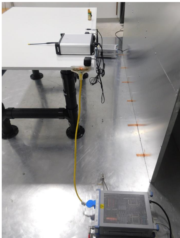
Figure 8.2-4: Conducted emissions – from AC mains power ports setup photo (SRX1200)
