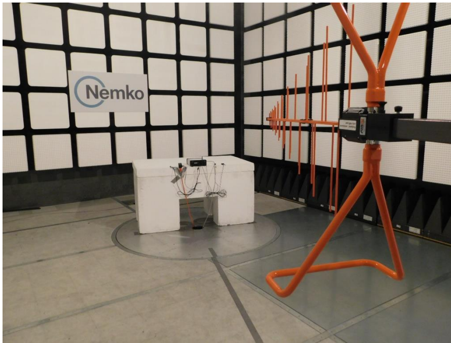
Figure 8.1-37: Radiated disturbance setup photo (SRX1200)
