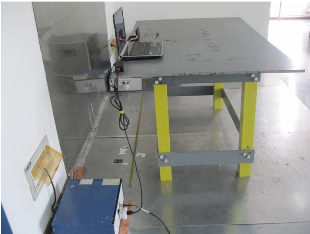
Conducted Emissions Test Setup - Side View
