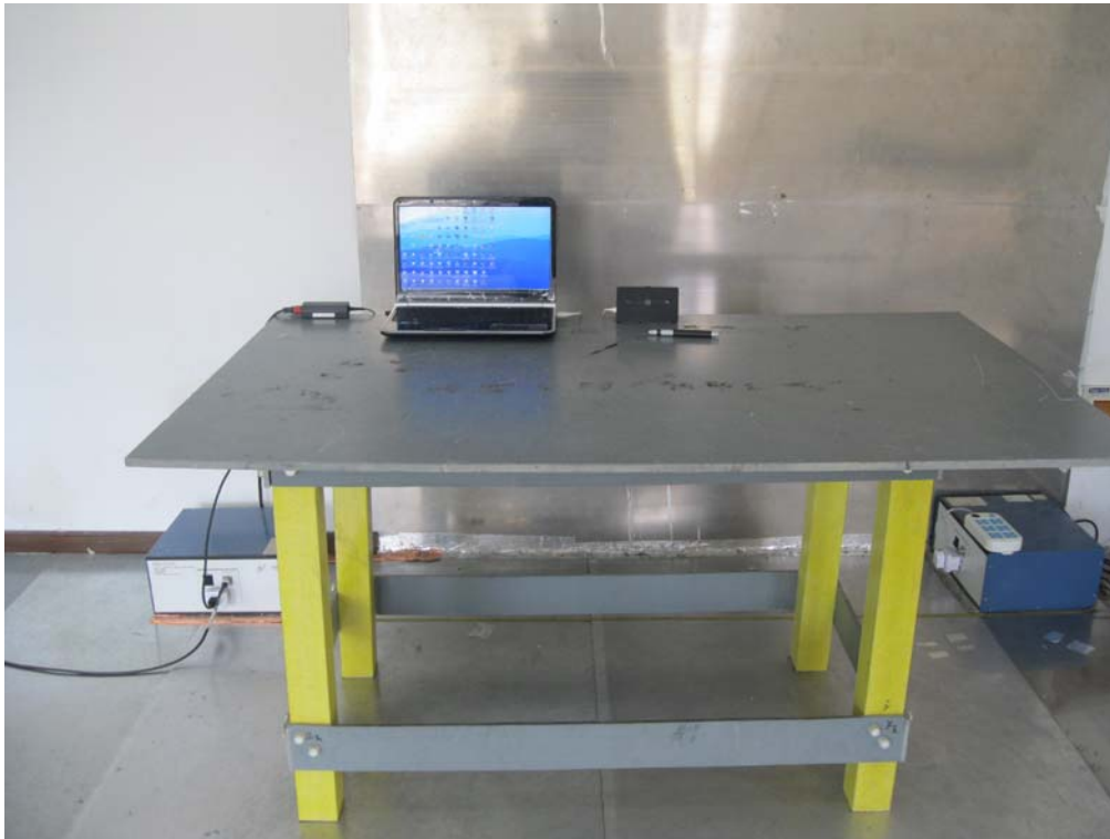
Conducted Emissions Test Setup - Front View
