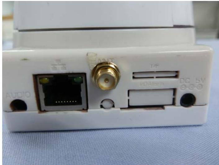
Equipment Antenna Connector: Reverse SMA Female
