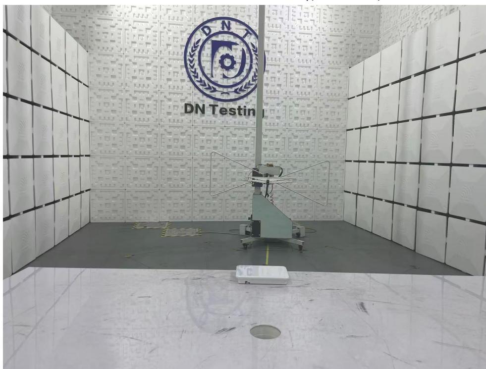
Radiated Emission Test View|(Below 1G)
