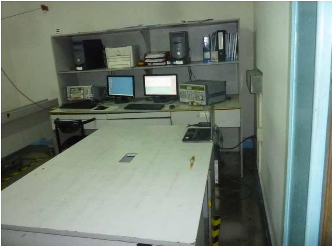
10.2.Photos of Radiated Emission Test (30-1000MHz)
