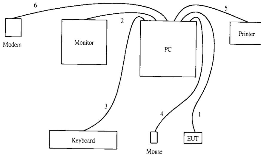
1. The I/O cable is connected from the support device 1 to the EUT.
