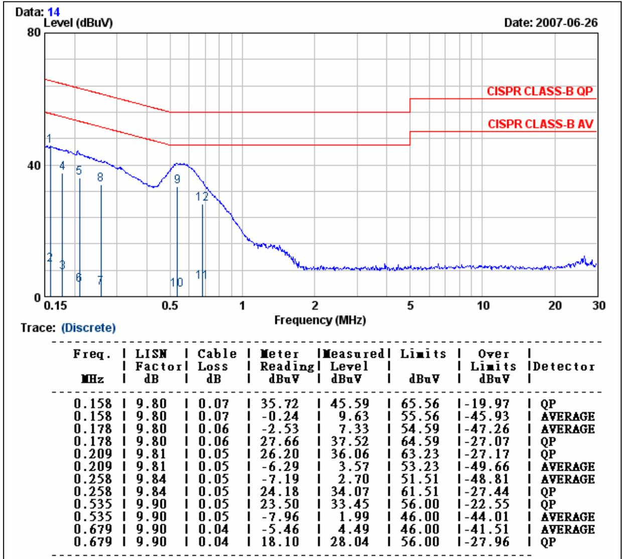
REMARKS : 1.Level (dBuV/m) = Read Level (dBuV) + Antenna Factor (dB/m) + Cable loss (dB)
