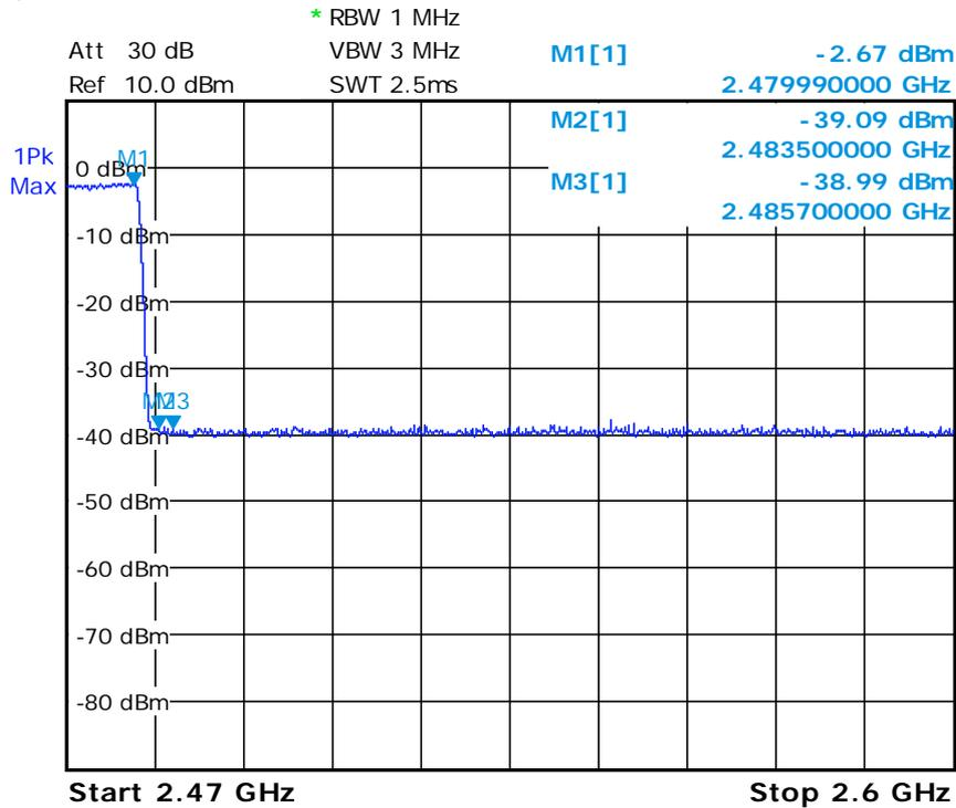
2. Radiated emission test :
