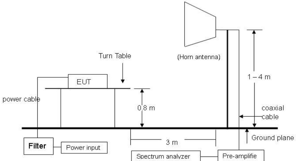
**NOTE :** The EUT system was put on a wooden table with 0.8m heights above a ground plane. For the actual test configuration, please refer to the photos of testing.
