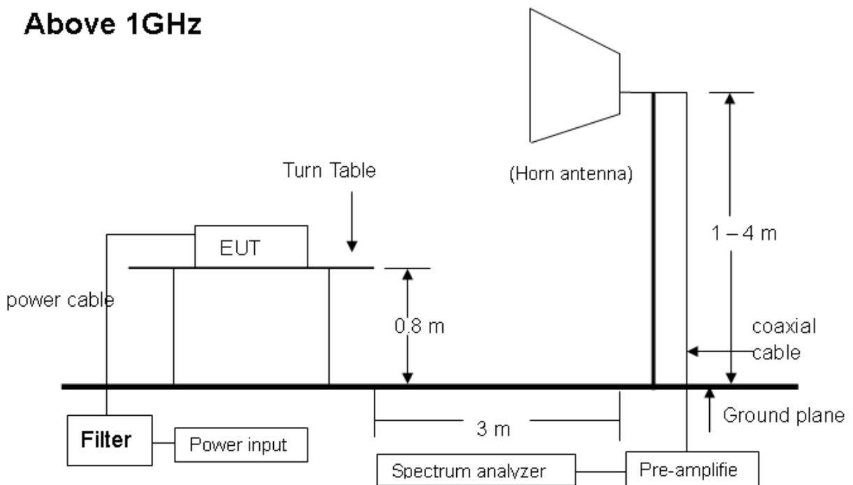
**NOTE :** The EUT system was put on a wooden table with 0.8m heights above a ground plane. For the actual test configuration, please refer to the photos of testing.
