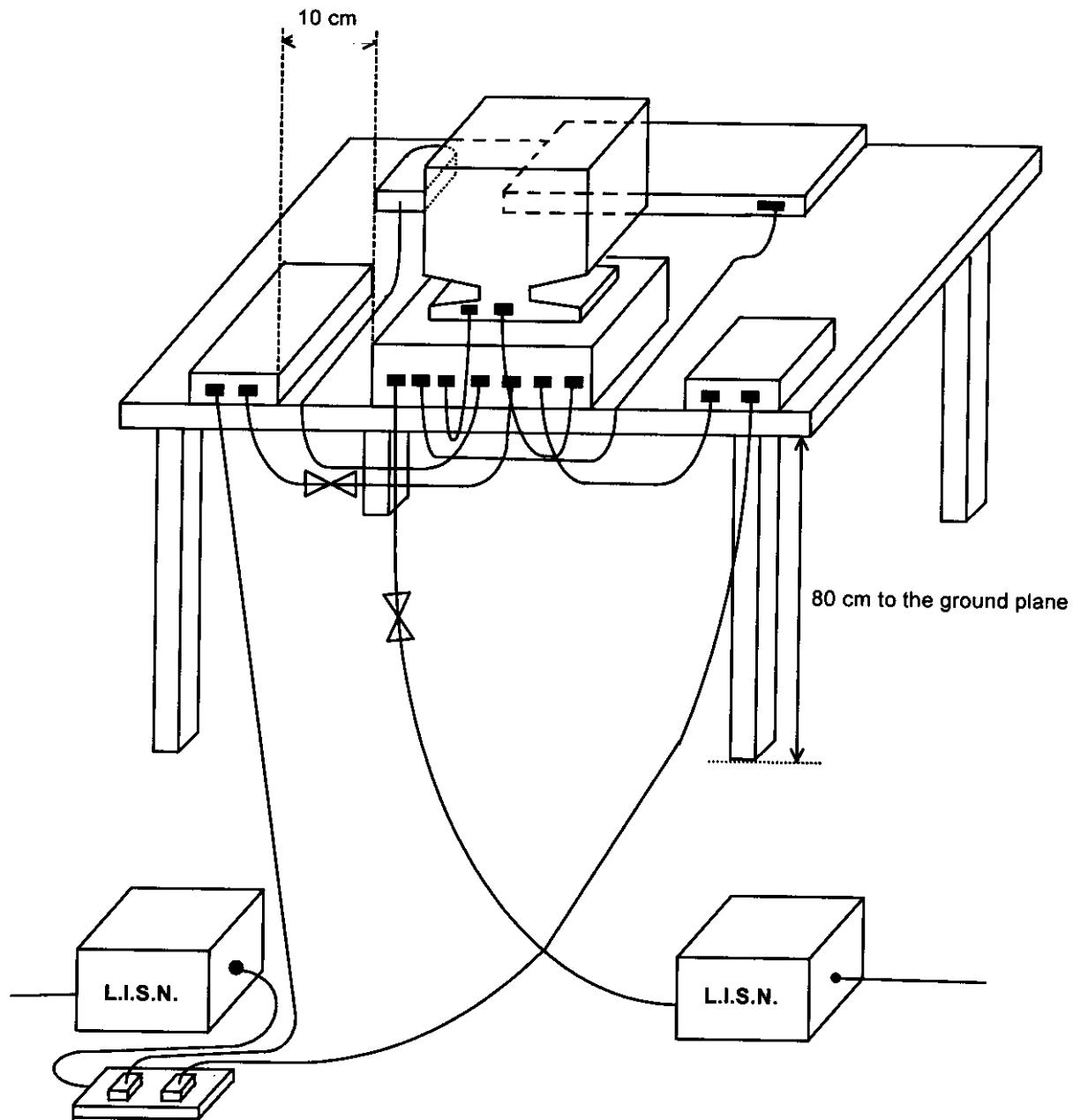
**5.4. Test Result of AC Powerline Conducted Emission****5.4.1. Test mode : 1600x1200 85Hz/106K (CRT Mode)**
