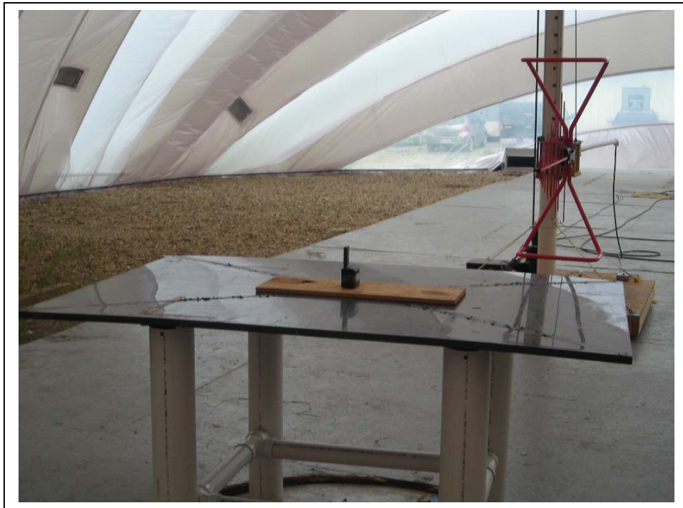
Pictorial 7: Radiated Emissions Test Setup – OATS E-Field Bilog Antenna, 3m Distance
