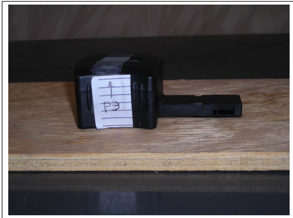
Pictorial 5: Radiated Emissions Test Setup – OATS Orthogonal Position 3
