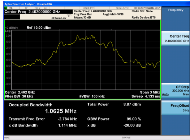
20dB Bandwidth plot on channel 39 (2Mbps)
