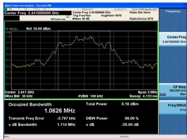
20dB Bandwidth plot on channel 39 (2Mbps)
