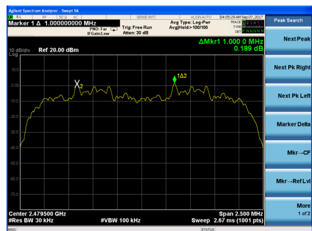
(2Mbps) Channel Separation plot on channel 77-78
