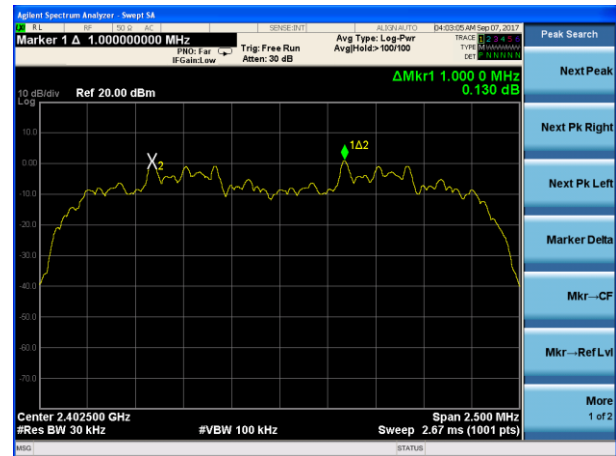
(2Mbps) Channel Separation plot on channel 39-40
