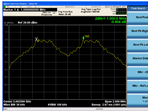
(1Mbps) Channel Separation plot on channel 39-40
