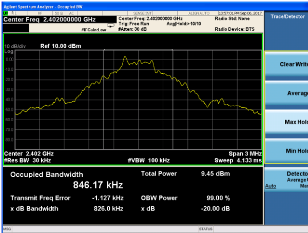
20dB Bandwidth plot on channel 39 (1Mbps)
