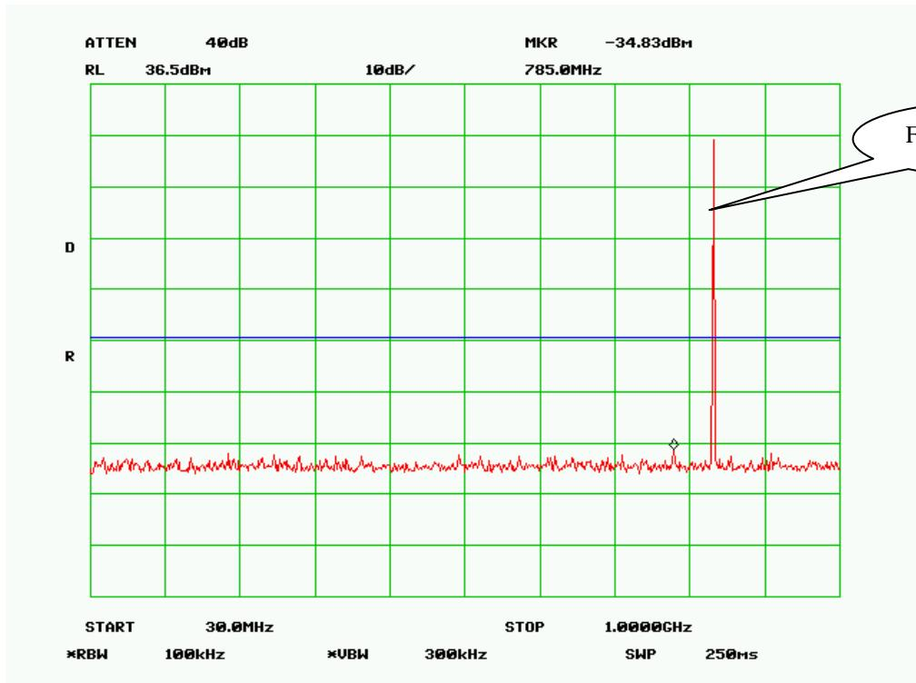
**1GHz-10GHz – GSM850 Middle Channel**
