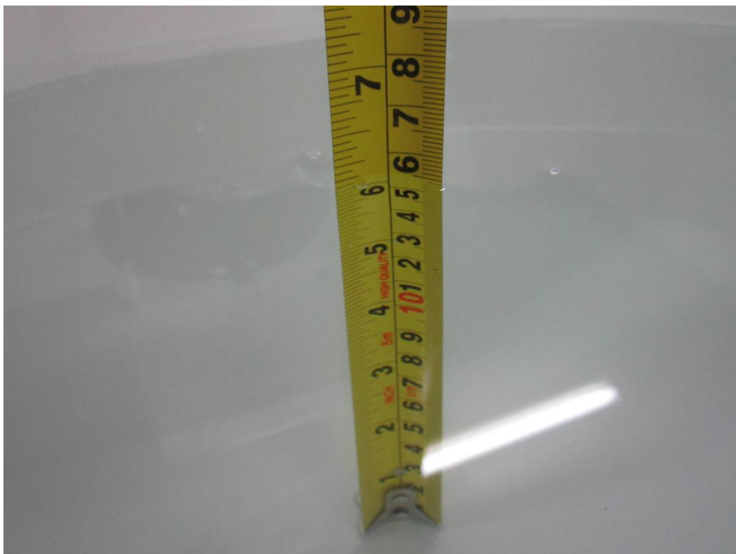
Liquid depth \geq 15\text{cm}
