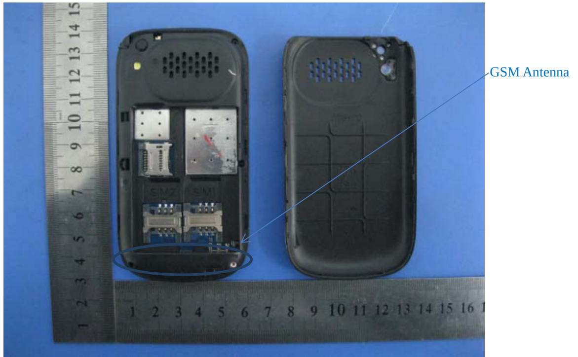
GSM Antenna - Top View
