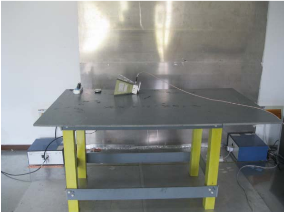
Conducted Emissions Test Setup - Front View
