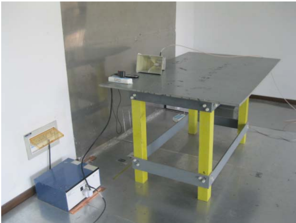
Conducted Emissions Test Setup - Side View
