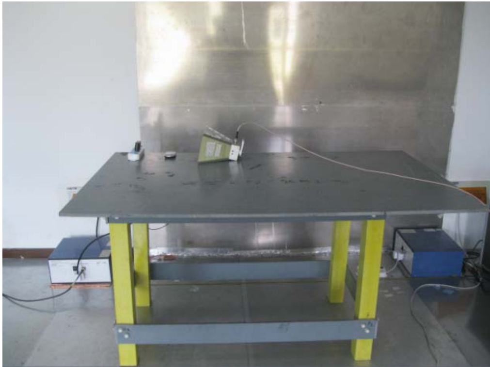
Conducted Emissions Test Setup - Front View
