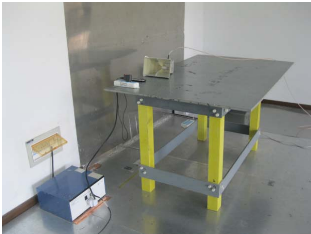
Conducted Emissions Test Setup - Side View
