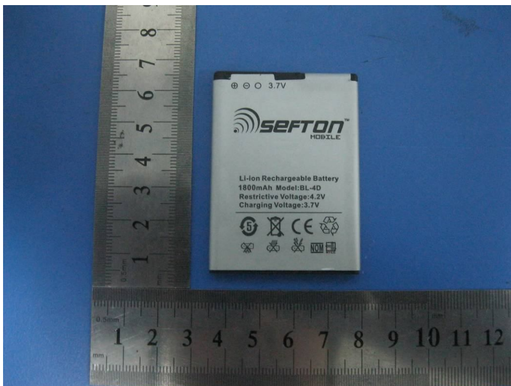
Battery - Top View
