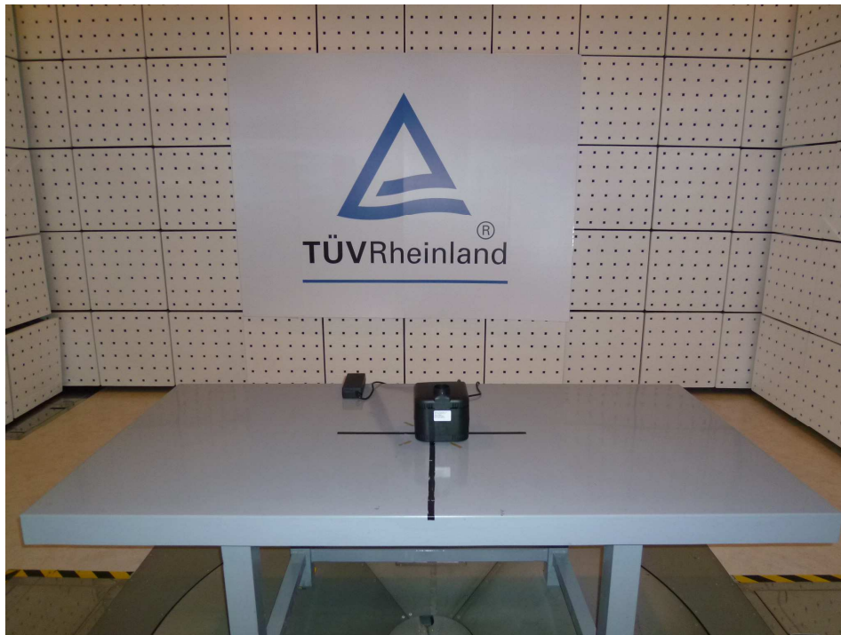
Photograph 1: Set-up for Spurious Emissions (Front View)
