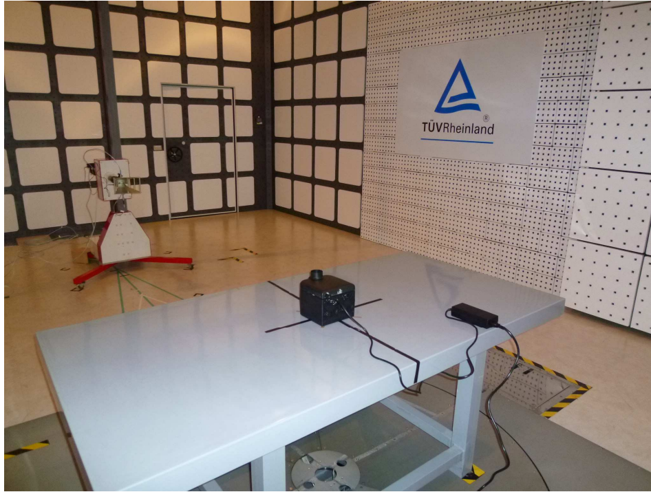
Photograph 3: Set-up for Spurious Emissions (Back View 2)
