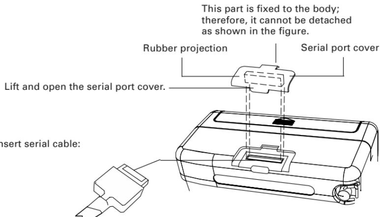
To replace the serial port cover, press in the rubber packing till the cover seats firmly.
