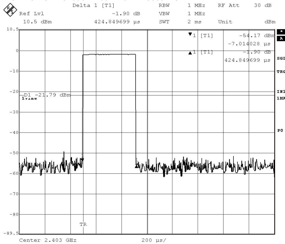
Mode of EUT : Hopping (DH3 packet) Max. power setting
