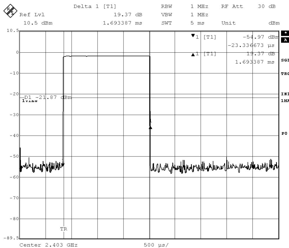
Mode of EUT : Hopping (DH5 packet) Max. power setting
