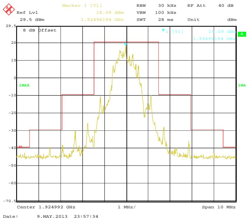
**High Channel (Unwanted Emission inside the Sub-band)**
