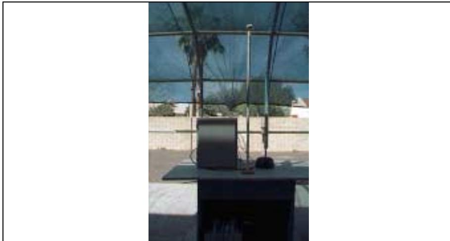
TEST SETUP: Radiated Emissions
