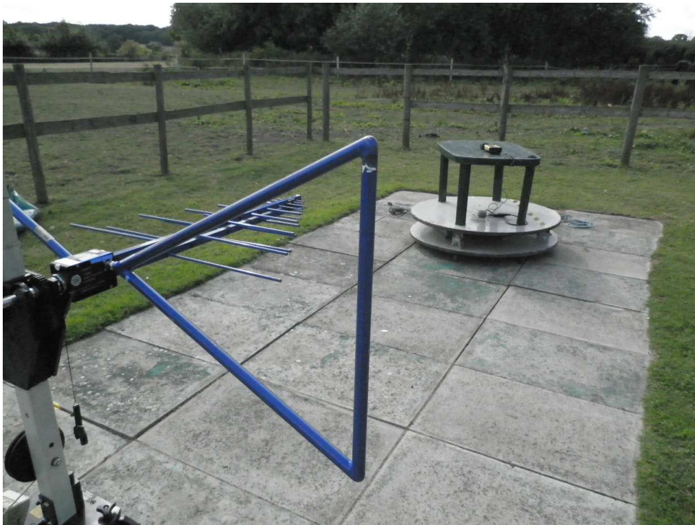
OATS 30MHz – 1GHz test set-up:
