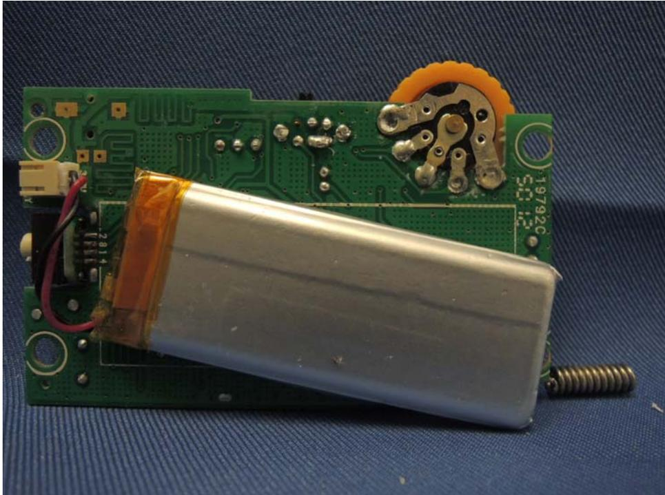
Baby Unit Main PCB solder side (View 2)
