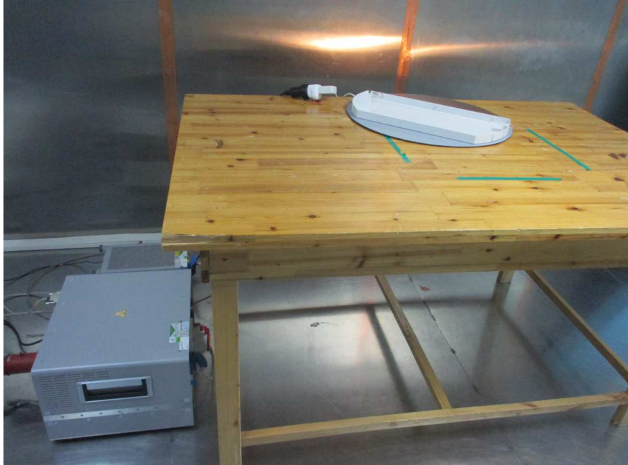
Photograph 1: Set-up for measurement of conducted emission
