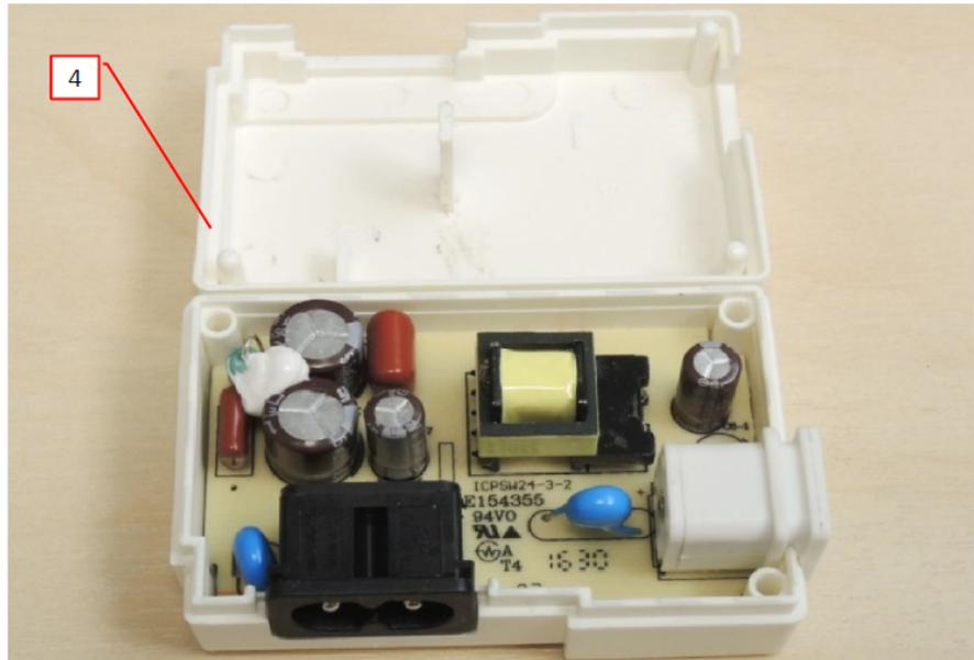
Photo 7 -External view of the PWB component side
