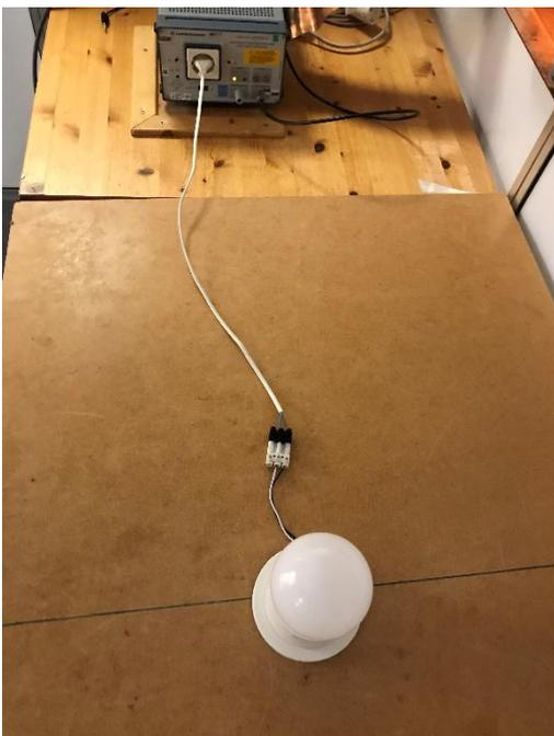
Test setup for conducted emission 150 kHz – 30 MHz
