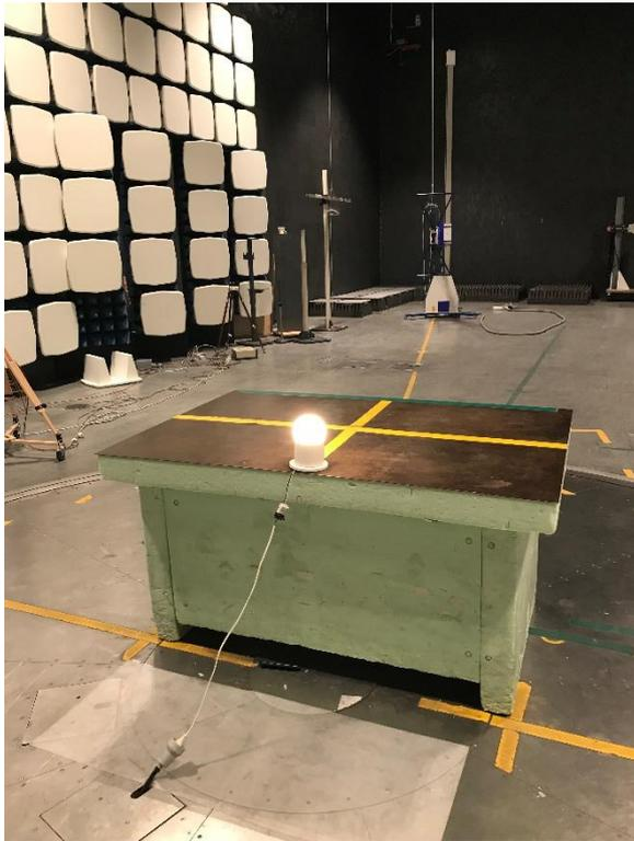
Test set up radiated emission 30 MHz – 1 GHz
