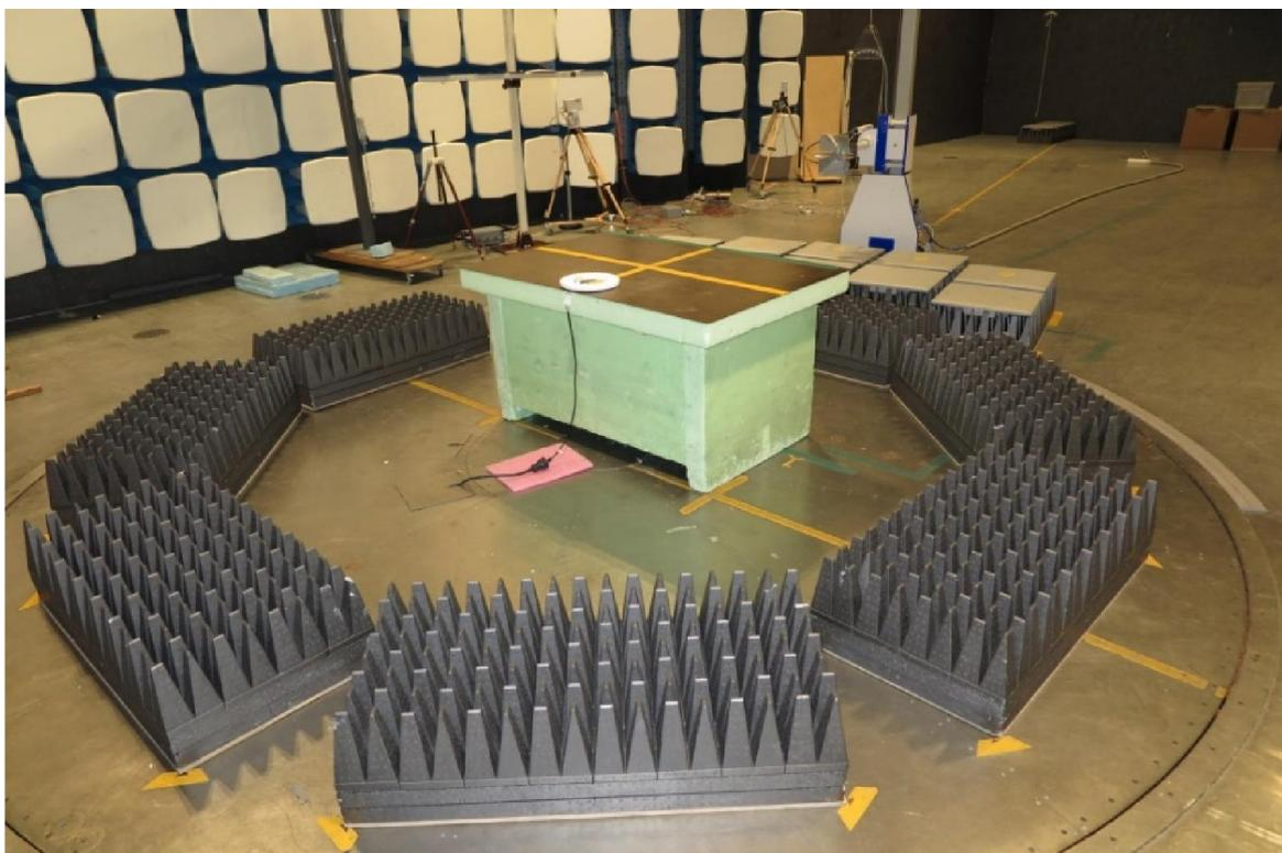
Test set up radiated emission 1 – 13 GHz
