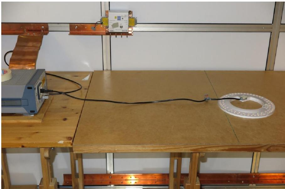
Test setup for conducted emission 150 kHz – 30 MHz
