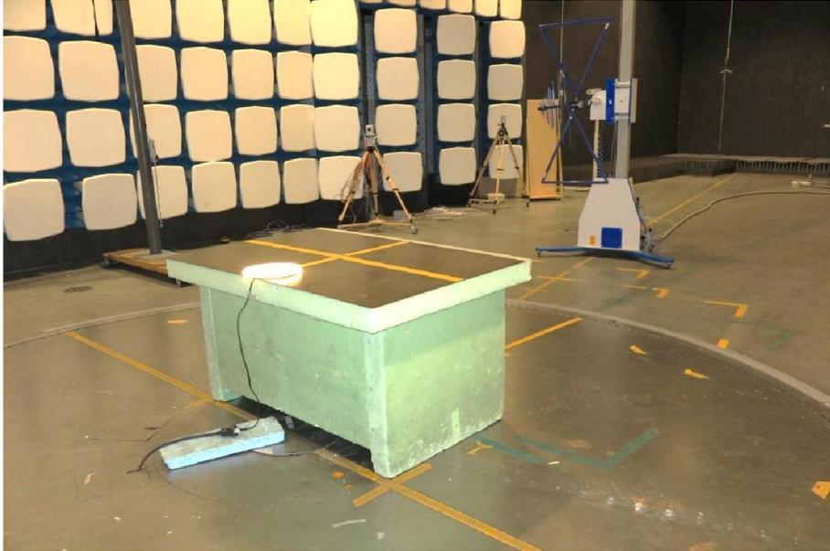
Test set up radiated emission 30 MHz – 1 GHz
