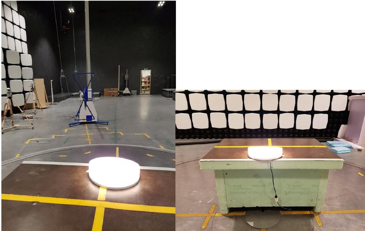
Test set up radiated emission 30 MHz – 1 GHz
