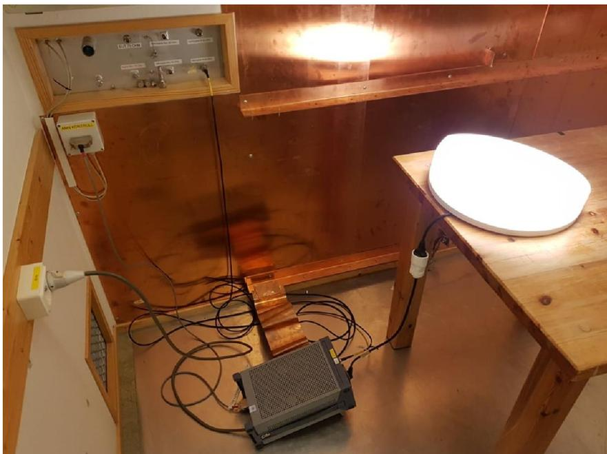
Test setup for conducted emission 150 kHz – 30 MHz
