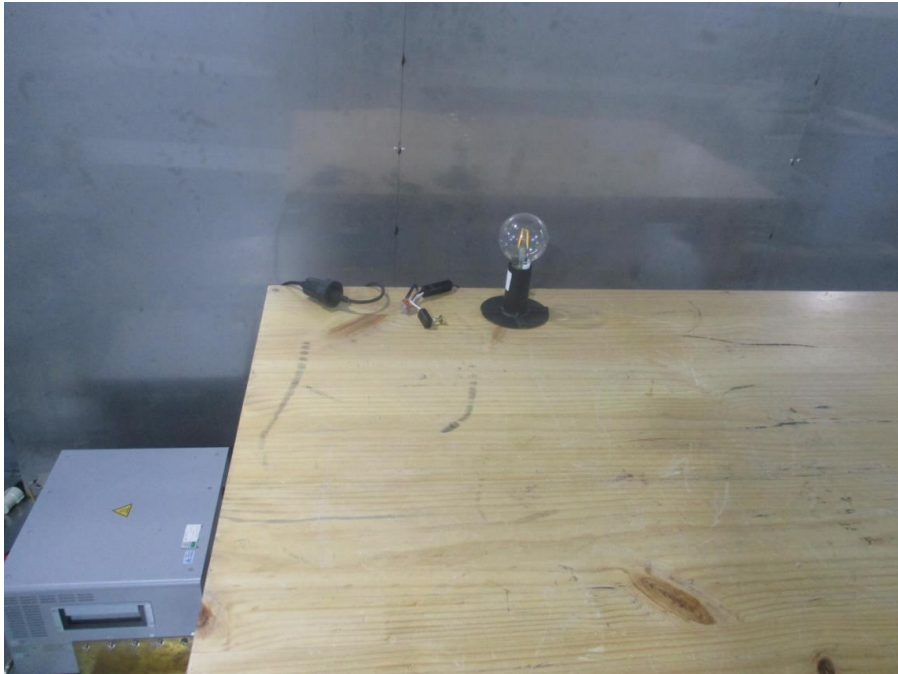
Photograph 1: Set-up for measurement of conducted emission
