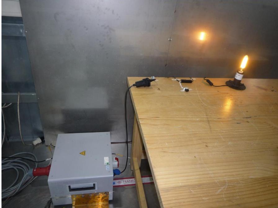
Photograph 1: Set-up for measurement of conducted emission
