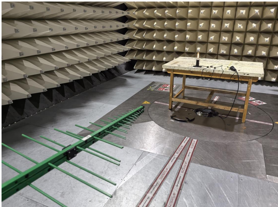
Photograph 2: Set-up for measurement of radiated emission
