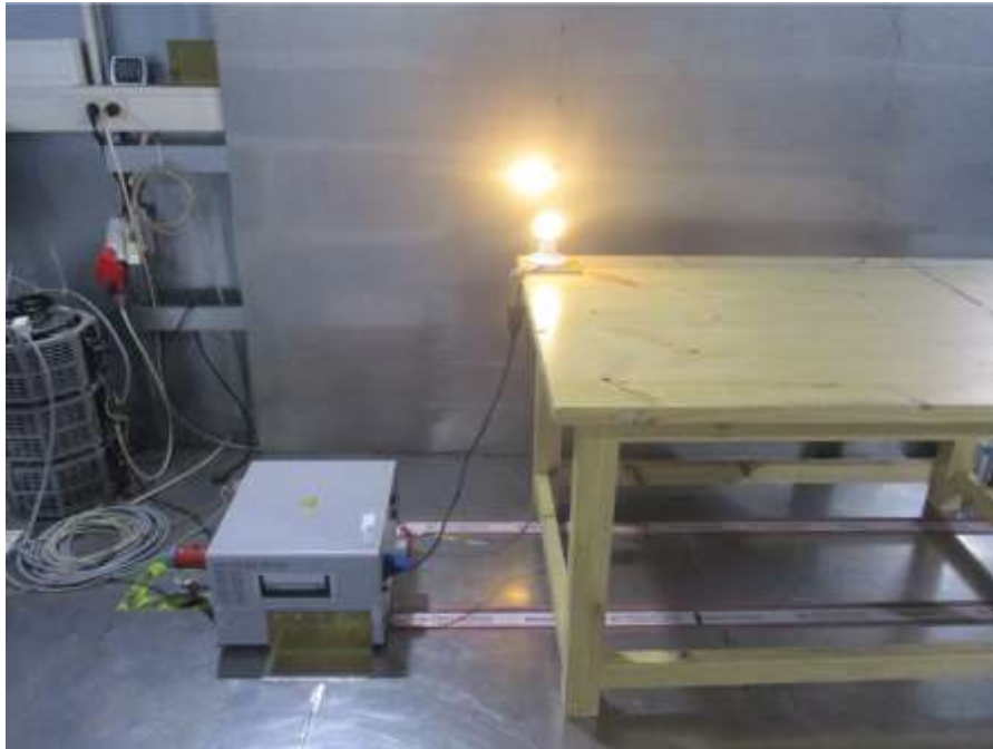
Photograph 1: Set-up for measurement of conducted emission
