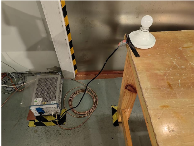
Photograph 2: Set-up for measurement of radiated emission
