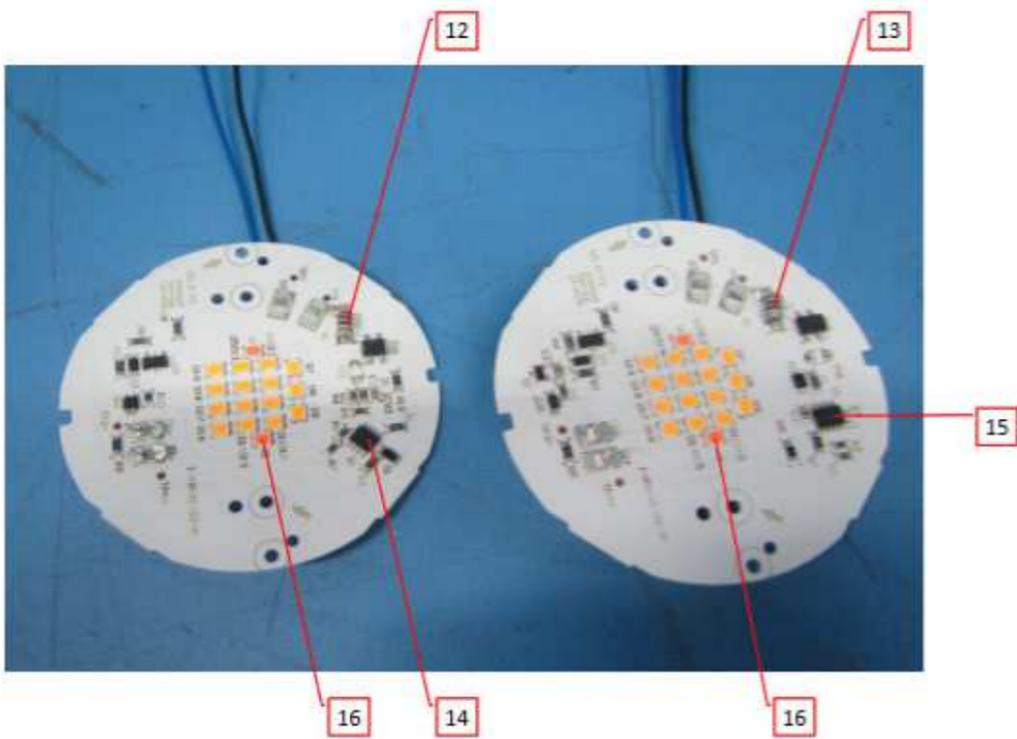
Photo 8 - Alternative driver PCB (Left - U1: BP5178FLD; Right - U1: SY59108N)
