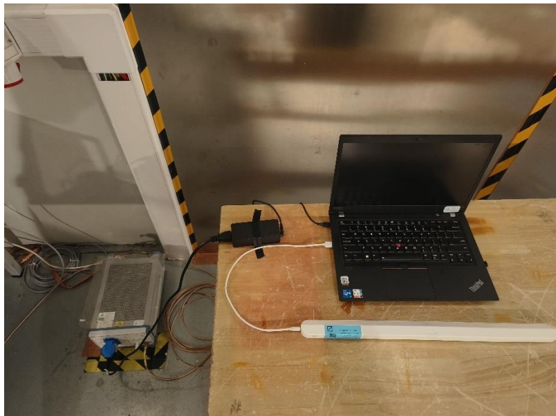
Photograph 2: Set-up for measurement of conducted emission, Mode 2
