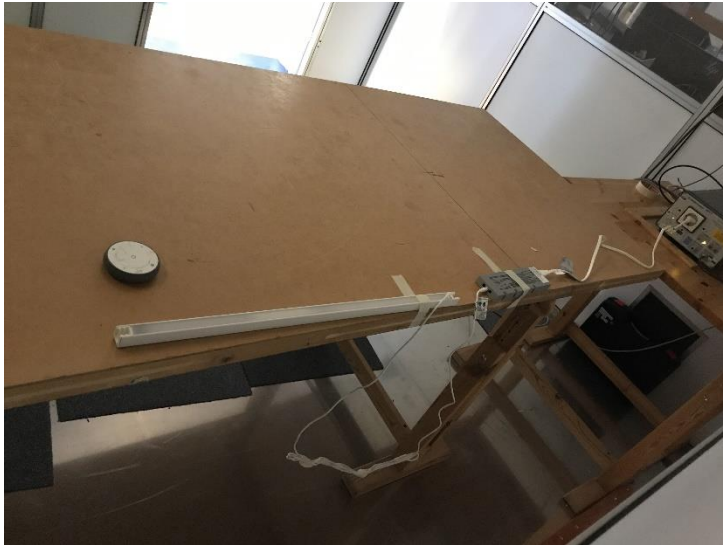
Test setup for conducted emission 150 kHz – 30 MHz, 10W
