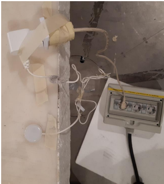
Test set up radiated emission 30 MHz – 1 GHz
