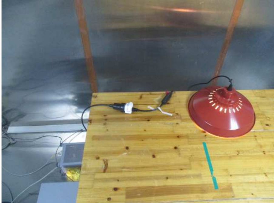
Photograph 2: Set-up for measurement of radiated emission
