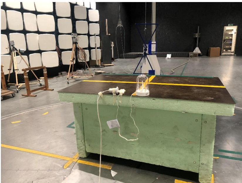
Test Setup for radiated emission, 30 MHz – 1 GHz, Charging mode
