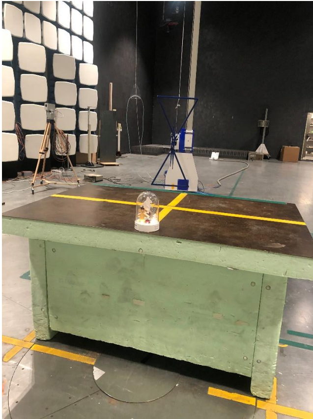
Test set up radiated emission 30 MHz – 1 GHz, battery operated
