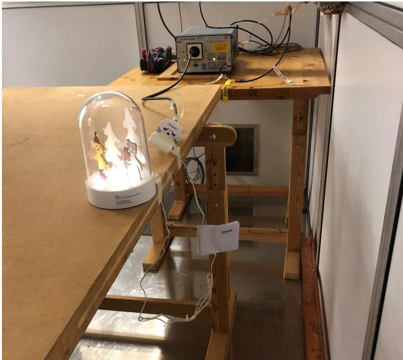
Test setup for conducted emission 150 kHz – 30 MHz
