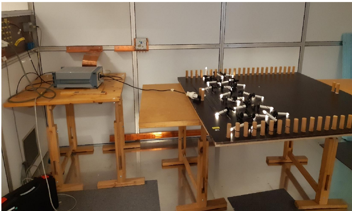
Test setup for conducted emission 150 kHz – 30 MHz
