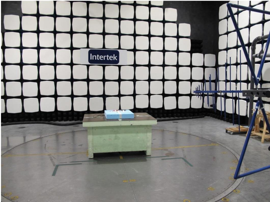
Test set up radiated emission 1GHz – 18 GHz
