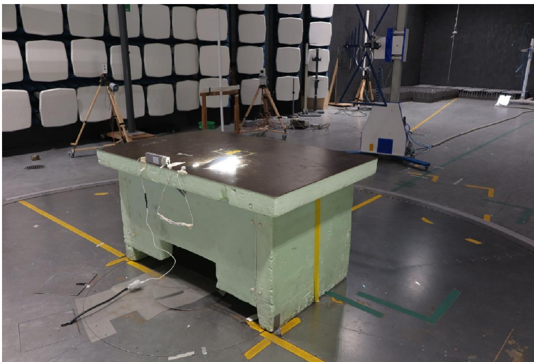
Test set up radiated emission 30 MHz – 1 GHz
