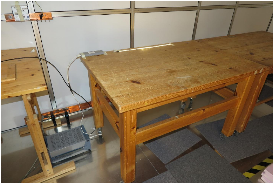
Test setup for conducted emission 150 kHz – 30 MHz
