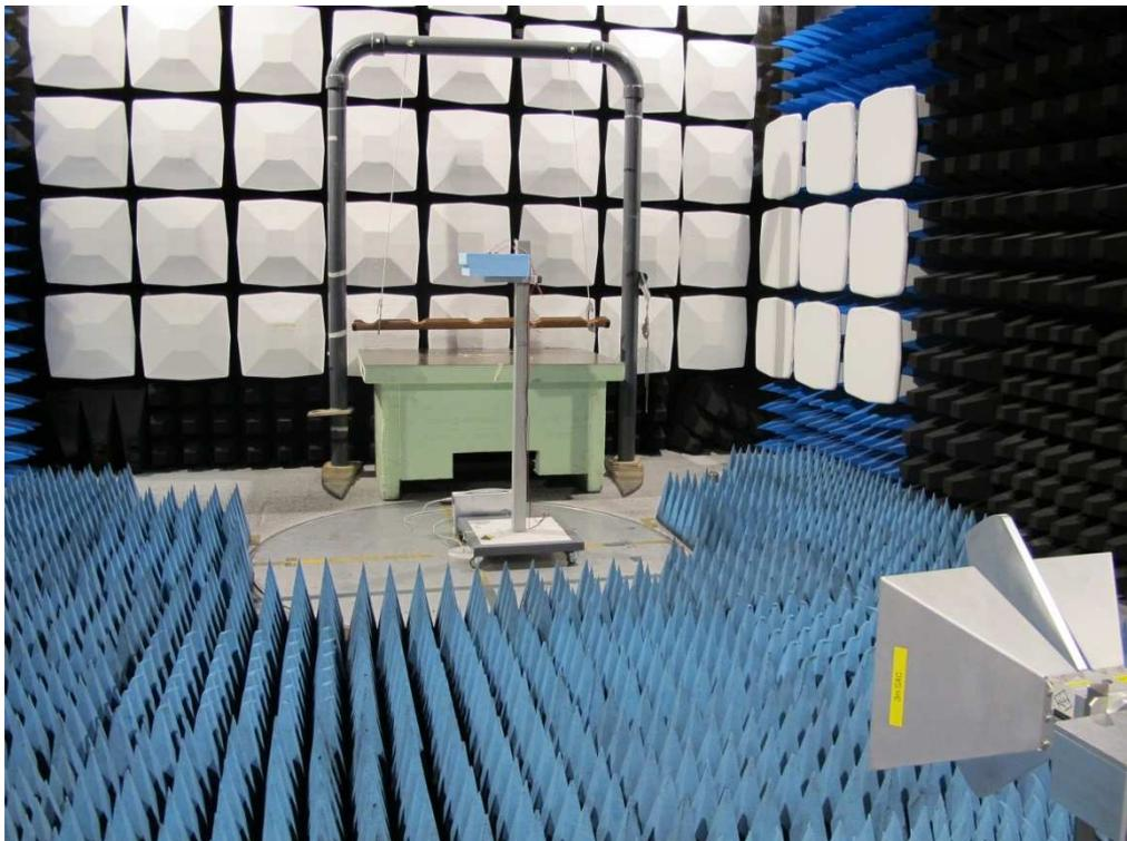
Test set up radiated emission 18 GHz – 26.5 GHz
