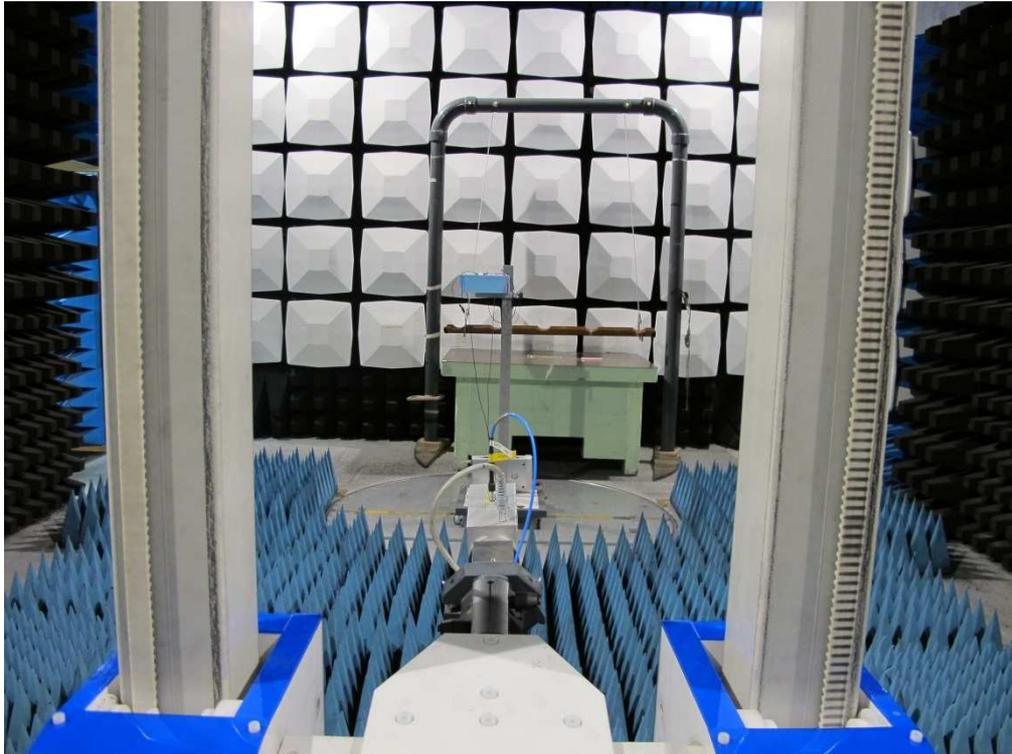
Test set up conducted emission 9 kHz – 30 MHz
