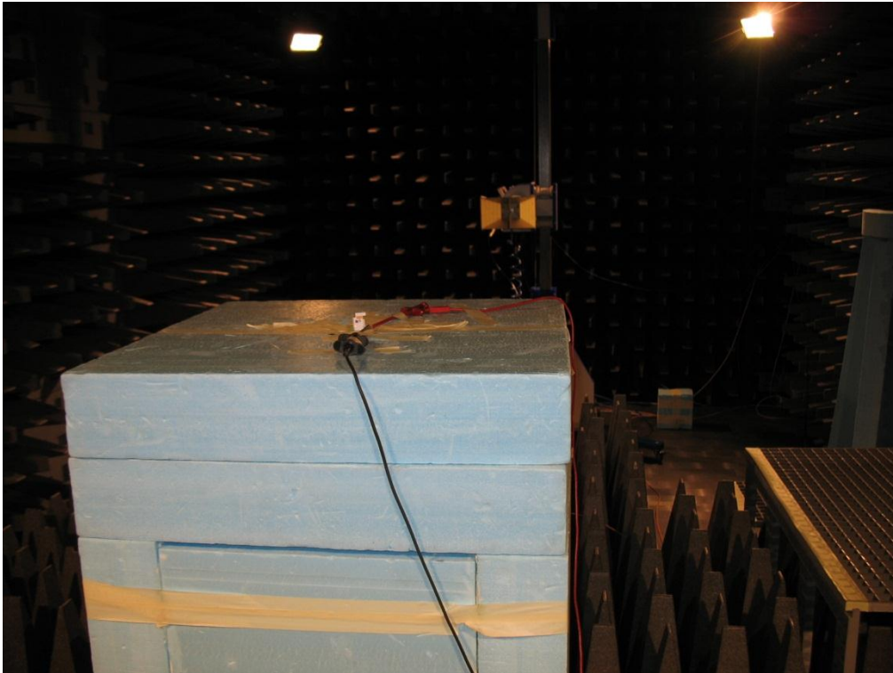
Test set up radiated emission preview sweeps 1 – 13 GHz, test site 'Wireless chamber'
