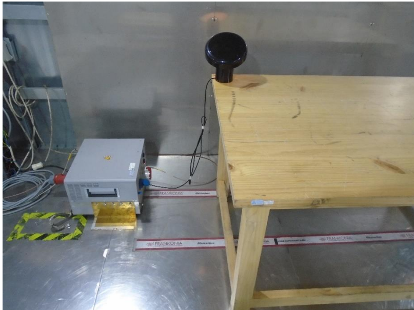
Photograph 2: Set-up for measurement of conducted emission
